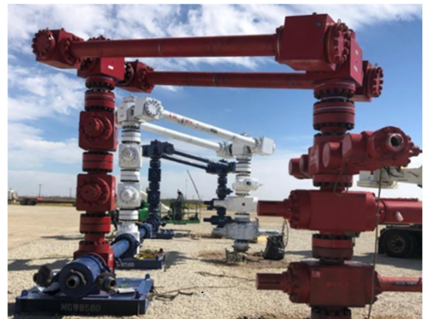
Zipper Bridge (no downlines required)
